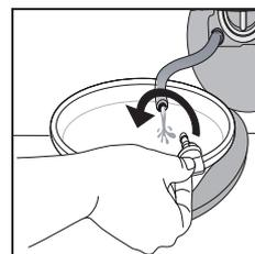
6. Turn the exhaust filter handle and pull it out of the housing. When the container is full with water, plug the stopper to the hose end, and reinsert the small hose in the washing machine's base. After, empty the container.
