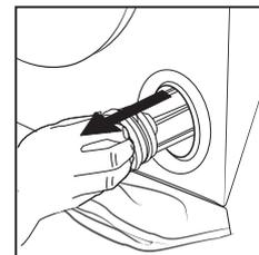
8. Clean the drain pump filter: remove residues in the filter and clean it under running water.
