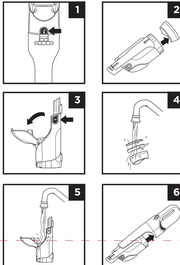
1. Press the dust cup release button and pull out the dust cup.
