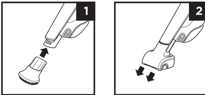
1. To attach an accessory, align it with the nozzle, then slide it on.
