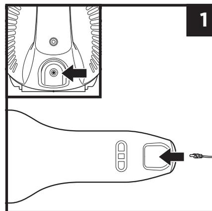
1. Insert the charging adapter plug into the port on the handle.
