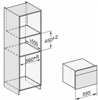
DG7x4x, DGM7x4x, installation drawings
