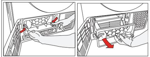
Clean the condenser by applying pressurized water with a shower armature and wait until the water drains.
