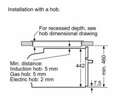
If the compact appliance will be installed underneath a hob, the following worktop thicknesses (including substructure if necessary) must be taken into account.
