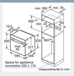
Installing two appliances on top of each other Air exchange
