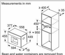
Bean and water containers are removed from the front Recommended installation height 950–1450 mm
