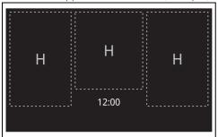
In both cases, the relative residual heat indicator disappears as soon as the temperature of a cooking zone falls below the safety threshold.
