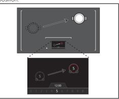
When you lift a pan, the appliance pauses all operations that are in progress (both cooking and timed cooking) and the pan is shown in arey on the display.
