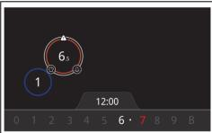
The pan with the highest power level (level 7 shown in red) is limited to the maximum level available (level 6.5 shown in white).
