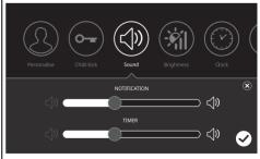
The "Notification" bar adjusts the volume of all sounds apart from the volume of the elapsed timer signal. The "Timer" bar only adjusts the volume of the timer sound signal. The far left end of a bar mutes the volume, while the far right increases the volume to the maximum
