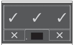
If a pan that is too large or non-circular is placed on the surface before it is switched on, it might be recognized as two separate pans. In this case, simply move the pan slightly on the surface or lift it and put it back down, until it is detected correctly.
