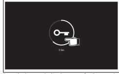
Press the key symbol in the centre for 3 seconds; an animation indicates that the display is being unlocked. The display is now unlocked.
